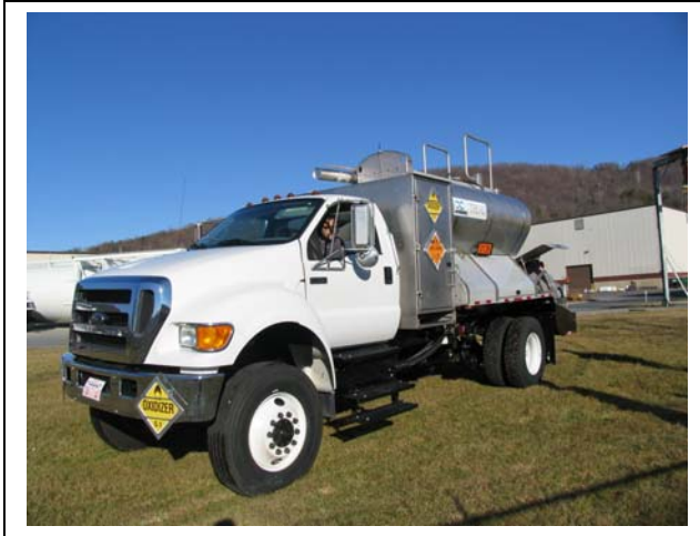
2009 UniBody 2607 Minipumper, SN3006 Mounted on 2008 Ford F750 4x4 chassis (This unit is not Canadian Compliant)
